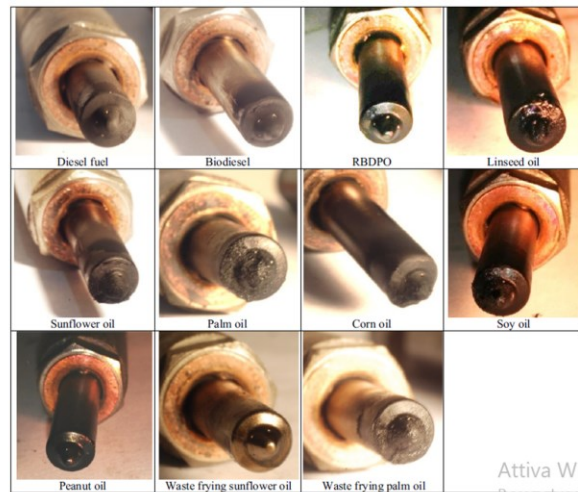
Fig. 9. Photo of the second injector after each test.
